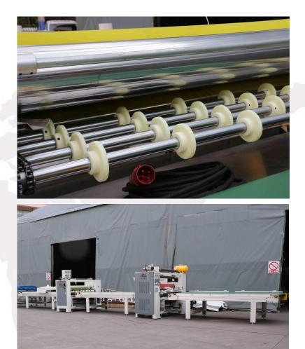
This machine is specialized for lamianting the transparent arylic sheet with the thin PVC, it can make many diffence patten, colour acrylic sheet.
